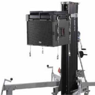
10. Now connect the first cabinet to the grid using CSSG ropes.
